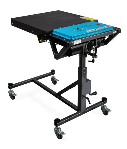
These versatile freestanding flash curing units are easy to use and easy to move. With quick flashing quartz elements and casters for easy maneuverability you can quickly move from garment to garment, increasing production.
