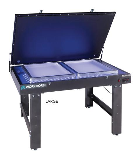
These tabletop and standalone units deliver fast exposure times and fine line detail using long lasting LED light strips. They will reduce your setup times, energy costs and overall cost of ownership. The LED strips operate at much lower temperatures, can last over 50,000 hours and start and stop immediately with the touch of a button.
